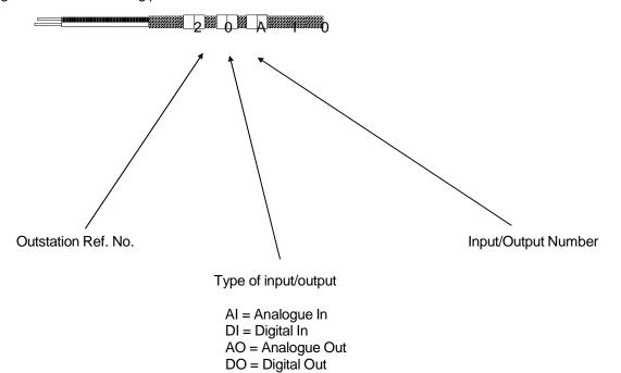
**N.B.** Multi-pair cables will require an overall identification Ref: on the outer sheath, using appropriate size heat shrink markers. Reference to be as per tender drawings.
